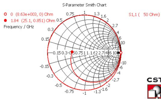
Figure 4. Smith Chart of Rectangular Microstrip Patch Antenna
