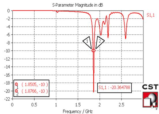
Figure 10. Simulation of Return Loss  $S_{11}$  and Impedance Bandwidth of RMPA with Proposed Metamaterial Structure
