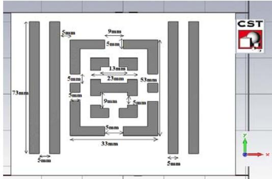
Figure 5. Design of Proposed Metamaterial Structure
