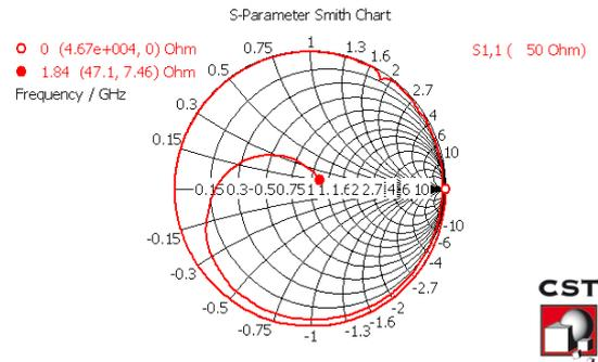
Figure 12. Smith Chart of RMPA with Proposed Metamaterial Structure
