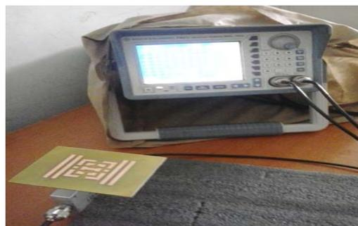
Figure 15. Setup for Measurement of Antenna Parameters
