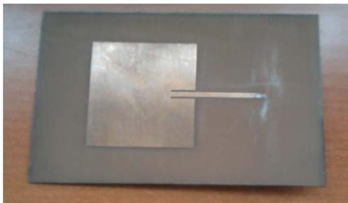
Figure 13. Fabricated Rectangular Microstrip Patch Antenna on PCB
